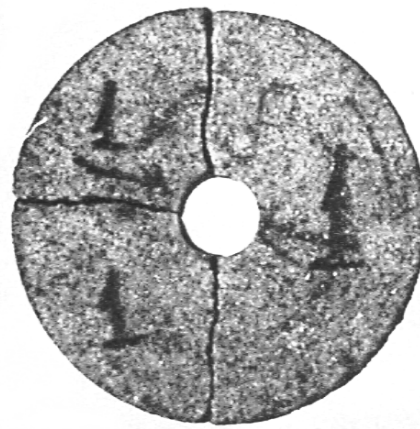
Figure 4: The ring specimen containing a horizontal pre-existing crack, destroyed by two vertical symmetrical cracks developing along the diameter.
