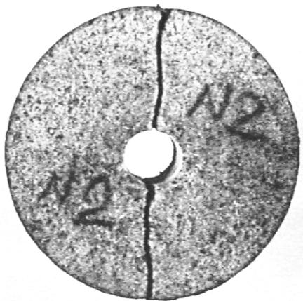
Figure 3: The ring specimen after the test. Two vertical symmetrical cracks have developed beginning at the edge the hole along the diameter in the applied force direction.
