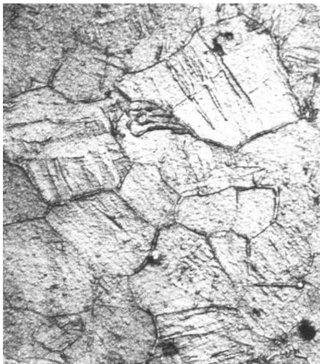
Fig. 6. Optical photomicrograph of AZ31B after being deformed in plane strain compression to 18% strain. Note the profuse amount of twinning.
