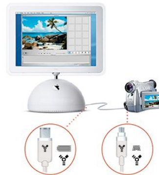
Figure: Connecting the 4-pin end to your camera, and the 6-pin end to the MAC.
